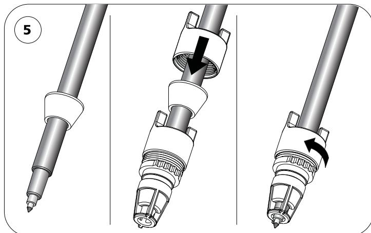
**5.** If the pen is not tight in the Pen Holder, pull the pen out and select a Rubber Collet that snugly fits the pen. (For an especially thin pen, the smallest Rubber Collet may be used.) Unscrew the Pen Holder Cap and remove the Plastic Collet from the Barrel. Slide the selected Rubber Collet over pen and insert the pen into the Pen Holder. Slide the Cap over the pen. Tighten the Cap until the pen does not move at all in the Pen Holder.
