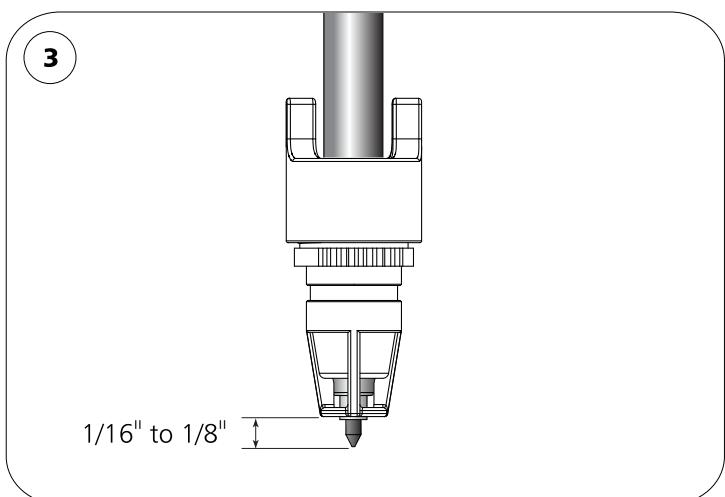
**3.** Tighten the Cap, ensuring that only  $1/16"$  to  $1/8"$  of the pen tip extends beyond the Pen Holder. If the pen tip extends beyond  $1/8"$ , the pen can mark material unintentionally as it moves across the material.
