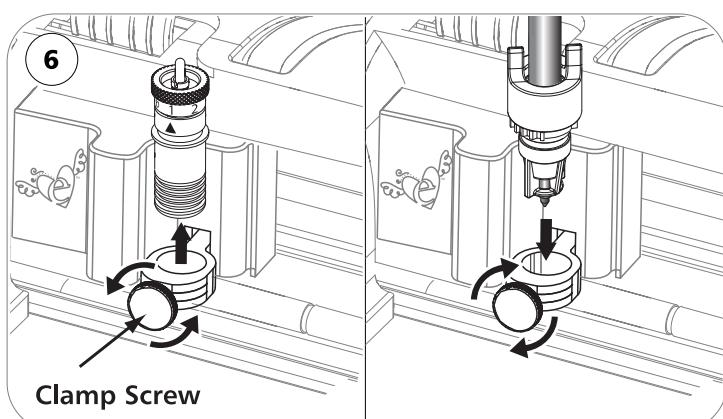
**6.** To install the Pen Holder in the eclips Machine, loosen Clamp by turning Clamp Screw counterclockwise approximately one full turn. Remove Blade Holder and place Pen Holder into Clamp. Tighten Pen Holder by turning the Clamp Screw clockwise until secure.
