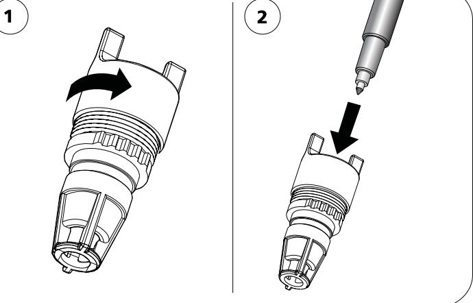
**1.** Loosen the Pen Holder Cap but keep it partially screwed onto the Barrel. The Plastic Collet is already installed in the Pen Holder.
